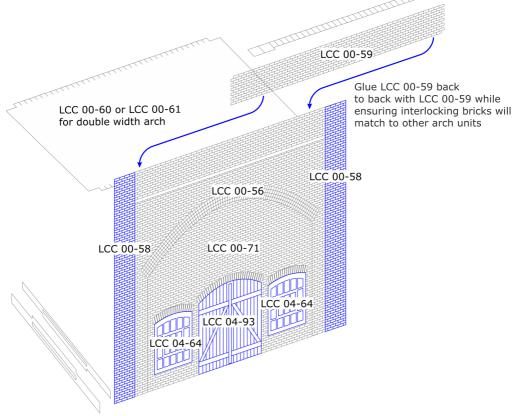
LCC 00-62 or LCC 00-63 for double width arch and use as bottom support to give the arch unit structural support
